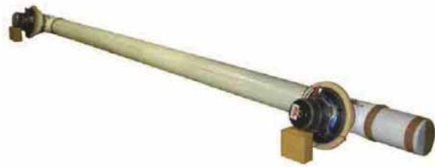
Figure 25: The acoustic enclosure used in sensor-less ANC experiment
