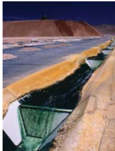
Figure 14: Collection of leachates from heap leaching (courtesy of CODELCO, Chile)
