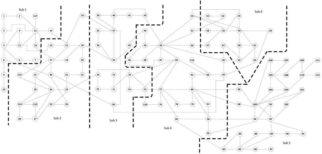
Fig. 6. Topological structure of the IEEE 118-bus system.
