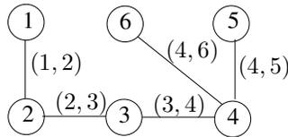
Fig. 7. The graph  $\mathcal{G}$  describing the partition of the IEEE 118-bus system.
