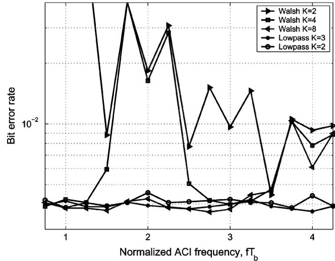
Fig. 4. Tolerance of Walsh and lowpass filtering methods to ACI.
