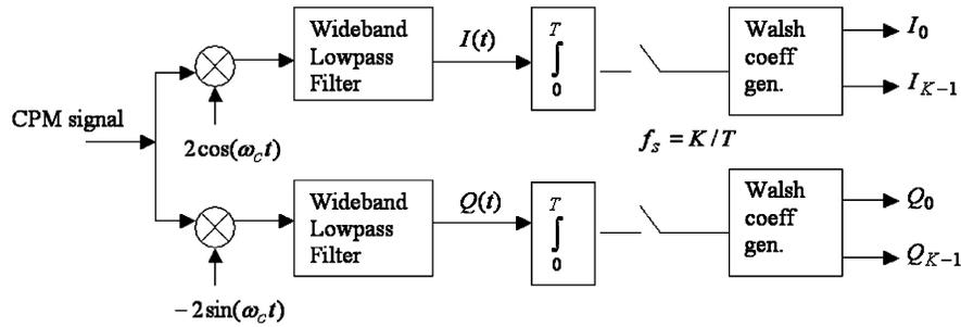
Fig. 1. Walsh filtering method for CPM Detection.
