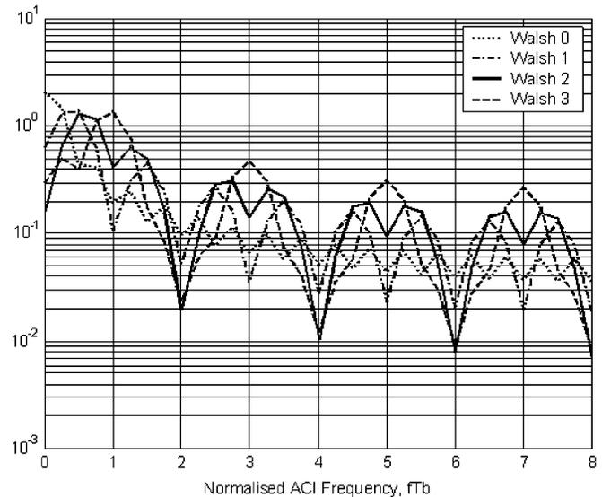
Fig. 3. Walsh coefficients as functions of ACI frequency ( $K = 4$ ).
