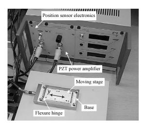
Fig. 1. Experimental setup of the PZT nanopositioner (The PZT actuator and position sensor attached to the moving stage are embedded into the base).
