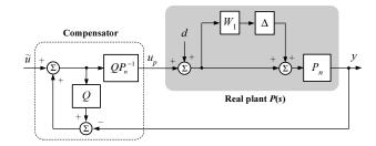
Fig. 4. Block diagram of inner-loop control system for hysteresis and resonance compensation.
