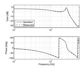
Fig. 3. Frequency responses of the PZT nanopositioner model P(s).
