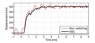
Fig. 10. Comparison of step responses between NSC and its non-switching case. The NSC is more effective to reduce the vibrations in steady state since a smaller gain is switched on when the output approaches the target.
