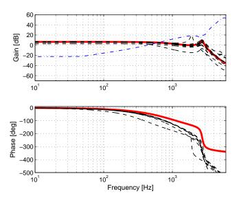
Fig. 5. Frequency response of nominal plant model  $P_n$ , perturbed plant models, and the relative uncertainty  $W_1$  used for design and analysis. (Solid thick line:  $P_n$ ; dashed lines: perturbed plant models; dash dotted line:  $W_1$ ).
