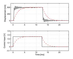
Fig. 8. Experimental results of repeated step tracking responses. The oscillations are almost removed with inner-loop compensator. The repeatability in the step responses indicates the robust performance of the compensator against the hysteresis with respect to various initial conditions. (Solid lines: Without compensator; dashed lines: with compensator)
