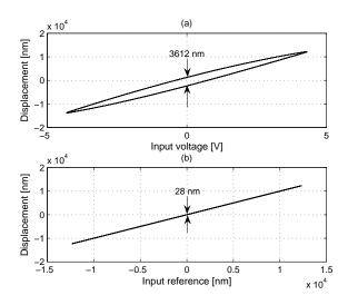
Fig. 7. Experimental results of hysteresis compensation. (a) Without compensator; (b) with compensator. The maximum gap between the hysteresis loop is significantly reduced from 3612 nm to 28 nm when the inner-loop compensator is applied.
