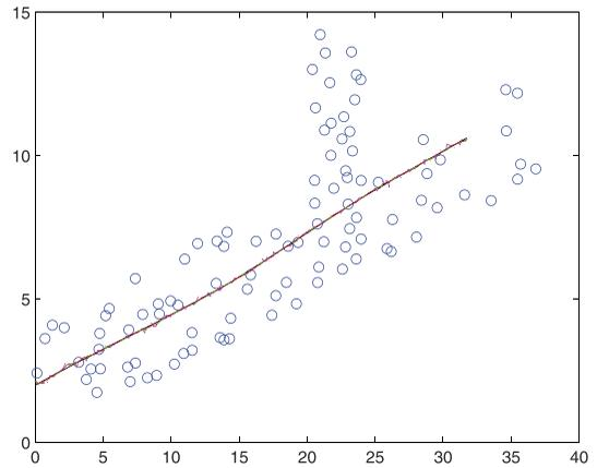
Fig. 8. The true and estimated trajectories of the target when it moves from A to C through B.
