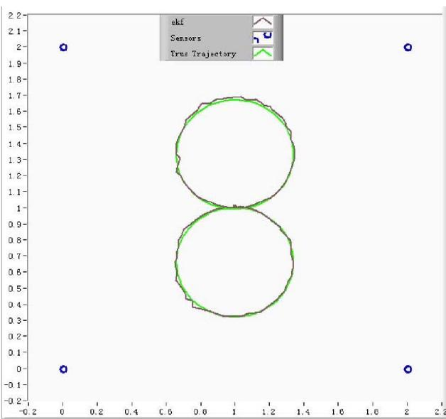
Fig. 3. Target tracking using extended Kalman filtering: The red line is the estimated trajectory using EKF, the green line is the programmed trajectory, and the four blue circles are sensor nodes.
