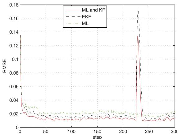
Fig. 7. RMSE of the three tracking approach when the target moves from A to B, then to D.
