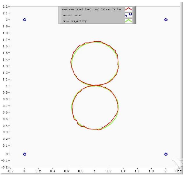
Fig. 2. Target tracking using proposed method: The red line is the estimated trajectory using the proposed method, the green line is the programmed trajectory, and the four blue circles are sensor nodes.
