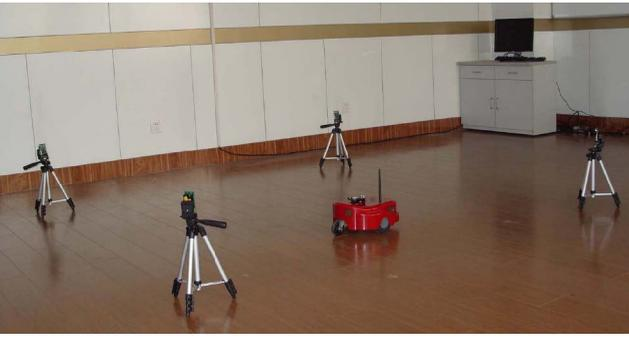
Fig. 1. Wireless sensor network testbed consisting of four sensor nodes, a base-station connecting to a PC, and a robot carrying a node as the moving target.
