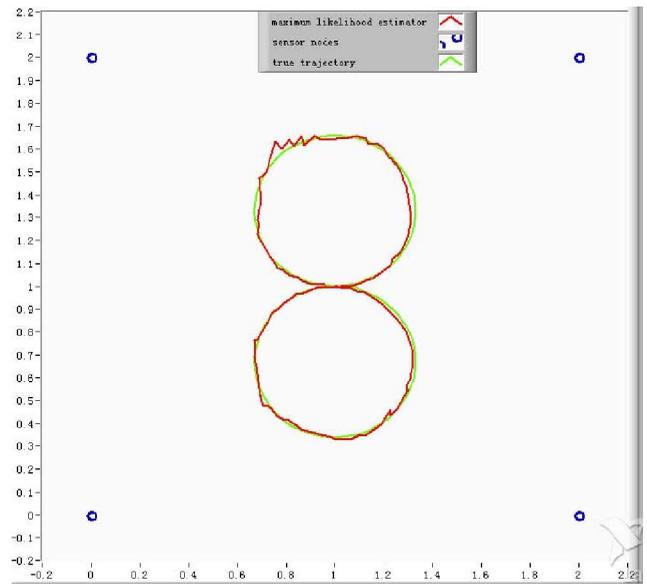
Fig. 4. Target tracking using maximum likelihood estimation only: The red line is the estimated trajectory using MLE only, the green line is the programmed trajectory, and the four blue circles are sensor nodes.
