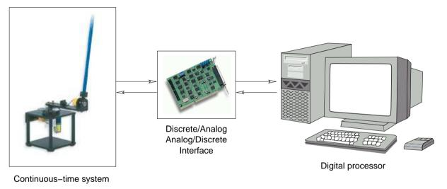
The continuous-time system, as seen from the discrete processor, is a discrete-time system.
