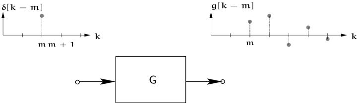
Then the output of the system to an arbitrary input sequence u[k] is given the discrete convolution
