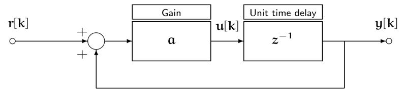
If the unit-sampling-time delay is replaced by its discrete transfer function  $z^{-1}$ , then the discrete transfer function from r to y can be computed as
