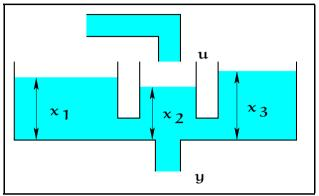
The controllability of the hydraulic system on the left is not so obvious, although we can see that  $x_1(t)$  and  $x_3(t)$  cannot be affected independently by u(t).
