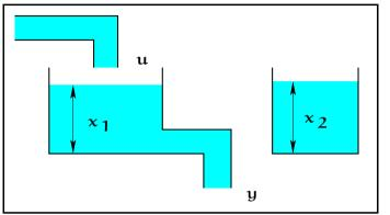
In the hydraulic system on the left it is obvious that the input cannot affect the level  $x_2$ , so it is intuitively evident that the 2-tank system is not controllable.
