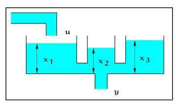
Now in the previous system suppose that the input is applied in the first tank, as shown in the figure. In this case the linearised model is the same as before, except that the matrix **B** is now different
