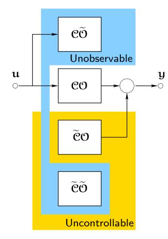
Every state-space equation can be transformed, by equivalence transformation, into a canonical form that splits the states into
