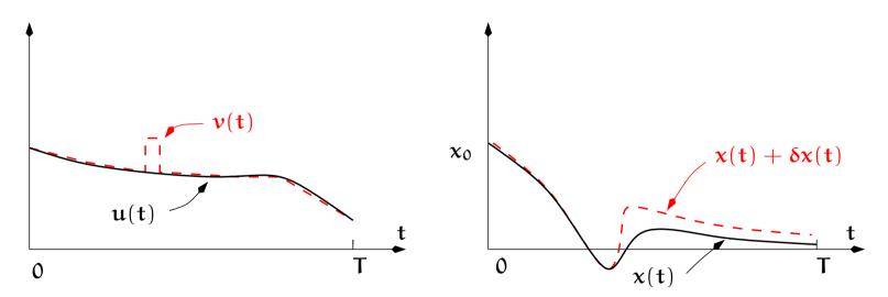
The input  $\mathbf{u}(t)$  generates the trajectory  $\mathbf{x}(t)$ . A variation  $\mathbf{v}(t)$  in  $\mathbf{u}(t)$ generates a different trajectory  $\mathbf{x}(t) + \delta \mathbf{x}(t)$ .
