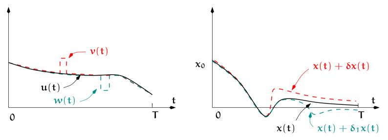
The input  $\mathbf{u}(t)$  generates the trajectory  $\mathbf{x}(t)$ . A variation  $\mathbf{v}(t)$  in  $\mathbf{u}(t)$ generates a different trajectory  $\mathbf{x}(t) + \delta \mathbf{x}(t)$ .
