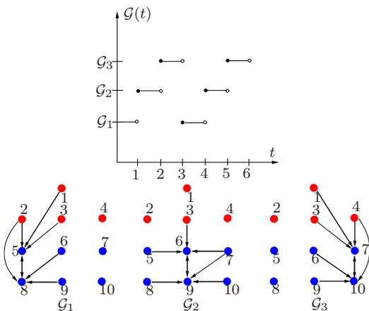
Fig. 5. A periodic switching graph  $\mathcal{G}(t)$  that switches among three different topologies.
