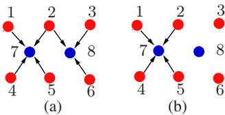
Fig. 3. (a) Sensing graph  $\bar{\mathcal{G}}$ . (b) Interaction graph  $\mathcal{G}$ .
