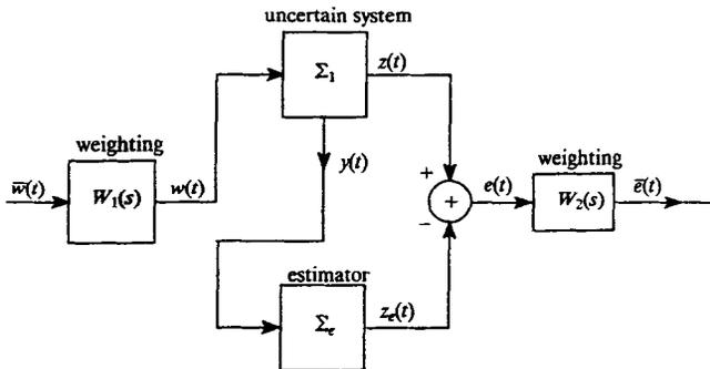
Figure 1. Block diagram of the robust estimation problem associated with system (1)
