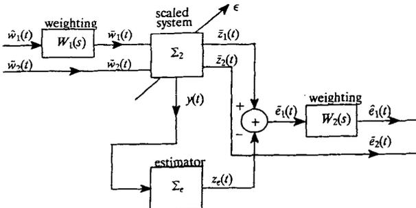
Figure 3. Block diagram of the scaled estimation problem associated with system (10)
