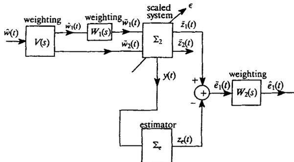
Figure 4. Block diagram of the scaled estimation problem associated with the interpolation approach
