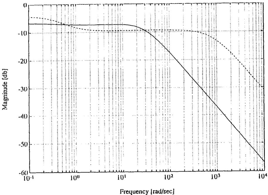
Figure 5. The estimation error spectra of the robust  $H_\infty$  estimator and the optimal  $H_\infty$  estimator based on the nominal system of (51) when  $f(t) \equiv 1$
